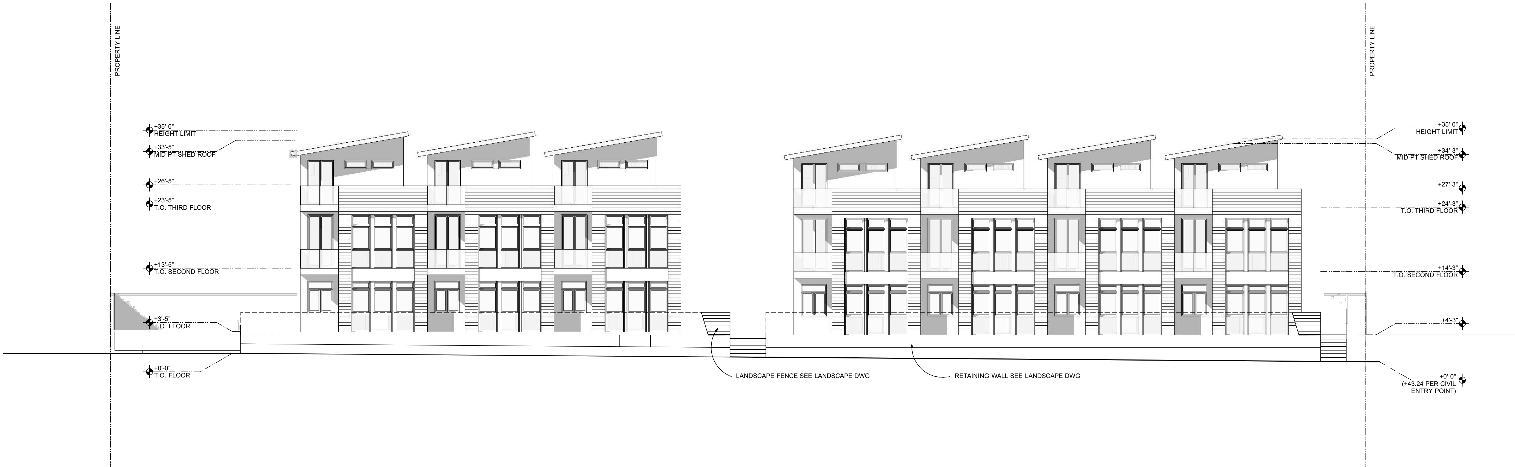
SELECTED DESIGN ELEVATION ALONG EL CAMINO REAL 1 SCALE 1/8"=1'-0"
